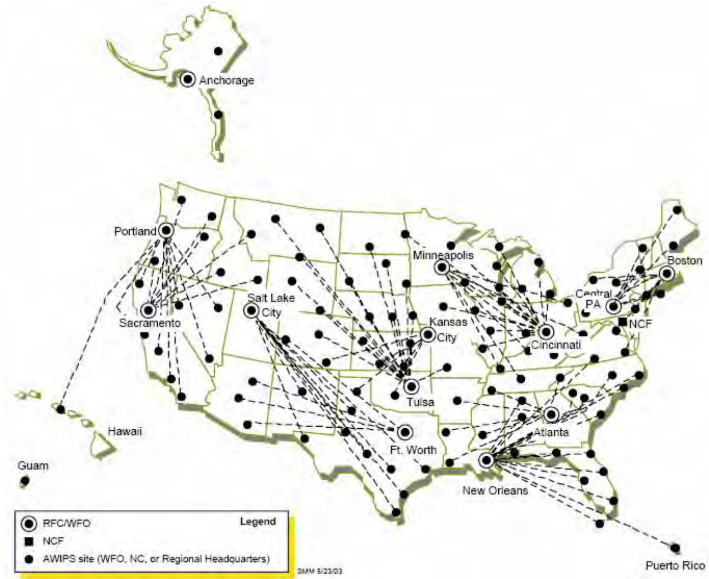
Exhibit 2.1.2-2. WFOs Connected to Alternate RFCs
