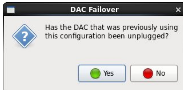
Exhibit 32.6-3 Confirm that the failed DAC is unplugged before proceeding
