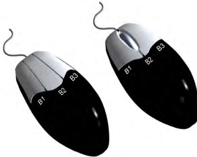
Exhibit 2.1.1-1. Right Handed Mouse (three-button mouse and a two-button mouse with clickable scroll-wheel)
